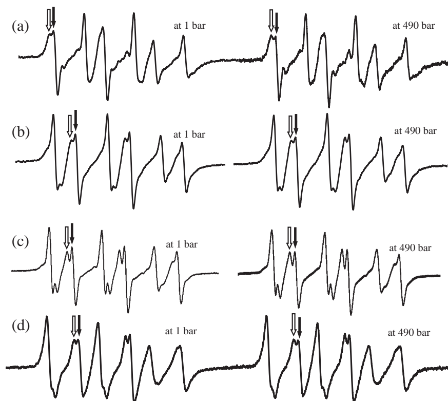
Fig. 8. ESR spectra of probes 1–3 in the presence of excess Calix- Sn under 1 and 490 bar at 290 K. (a) [ 1 ] = 2.5 \times 10^{-4} mol dm ^{-3} and [Calix-S8] = 8.0 \times 10^{-3} mol dm ^{-3} . (b) [ 2 ] = 2.5 \times 10^{-4} mol dm ^{-3} and [Calix-S8] = 7.0 \times 10^{-3} mol dm ^{-3} . (c) [ 2 ] = 2.0 \times 10^{-4} mol dm ^{-3} and [Calix-S6] = 1.5 \times 10^{-2} mol dm ^{-3} . (d) [ 3 ] = 2.5 \times 10^{-4} mol dm ^{-3} and [Calix-S6] = 3.2 \times 10^{-2} mol dm ^{-3} . Open arrows and closed arrows are assigned to the group-in complexes and free radical species, respectively.
